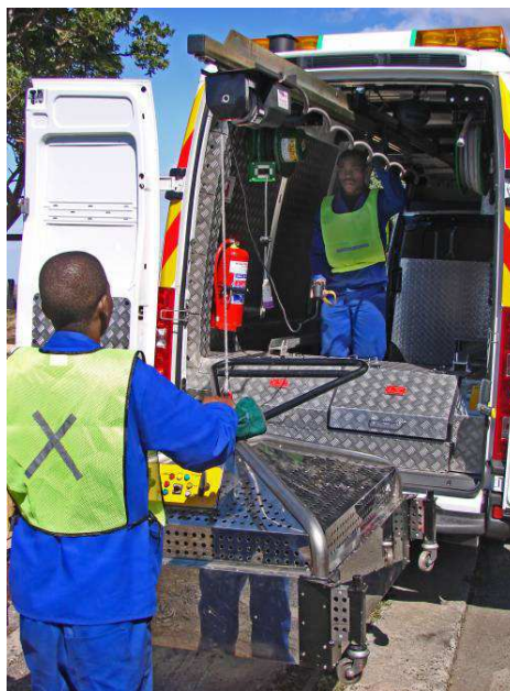
Removing infrared heater from rear of van using extended hoist
